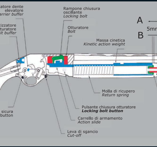
possible position to eject any ammunition. Chambering cartridges is easy thanks to a special free floating carrier that makes it possible to rapidly cycle ammunition just operating the bolt handle.
