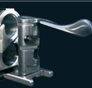
Since our actions are forged from solid billets, in either steel or light alloy, the material does not experience excessive cutting during machining. Therefore the actions are stronger and absorb recoil better. All our actions in NiCrMo are cemented and hardened to have a very flexible core and a very hard surface.
