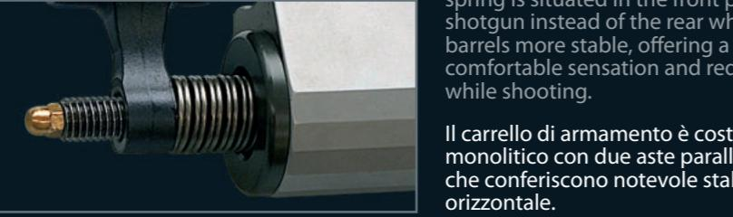
Inertia-operated semiautomatic shotguns offered by Caesar Guerini work with a special double disk spring (not a coil spring) located on the magazine in the front fore-end section. Should one of the components break, the shotgun would still operate.
