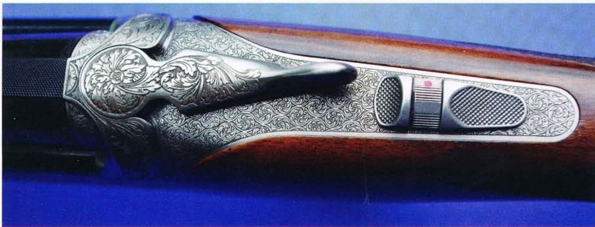
The barrel selector is part of the top-tang safety, with exquisite engraving also on the fences and opening lever.
