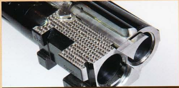
The jeweled monobloc showing its bottom locking lugs and the bite for the locking bolt. See also the disc retainer for the ejector
